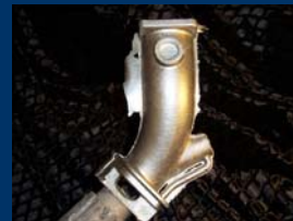
Pipe from a ZCast mold – this is an Aluminum Alloy
