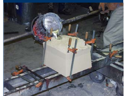
Direct pouring molten aluminum into a ZCast mold. The mold was printed on the ZCorp 310 3D printer.
