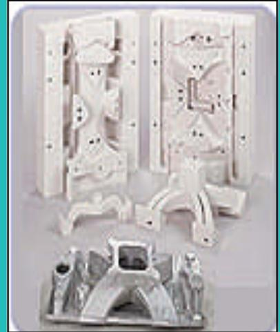
Above: Intake manifold and it's mould using Zcast technology.
